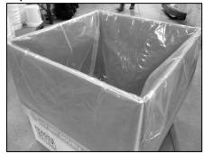
Add liner to box and fold over flaps of the box. Open liner into all four corners of the box to avoid bunching.
